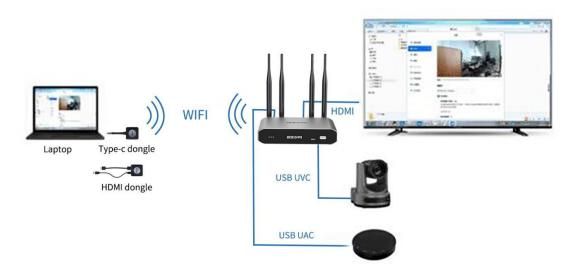
The USB conference camera is connected to the front USB port of the base unit, while the USB omnidirectional microphone speaker for meetings is connected to the rear USB port of the base unit. The HDMI OUT of the base unit is then connected to the display screen or projector.
